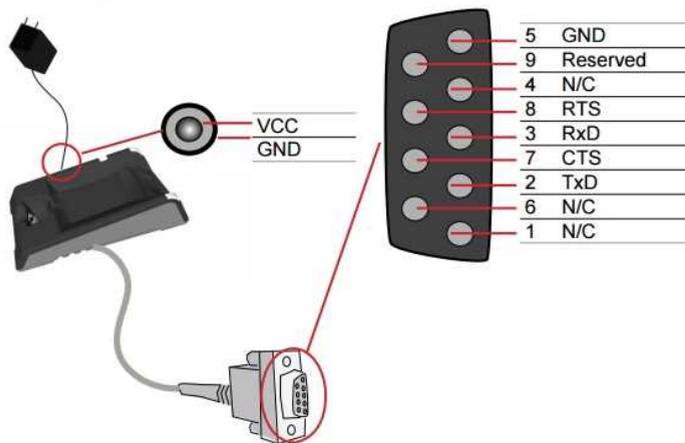
**WARNING:** For proper RS-232 operation, do not apply any voltage to pin 9.
