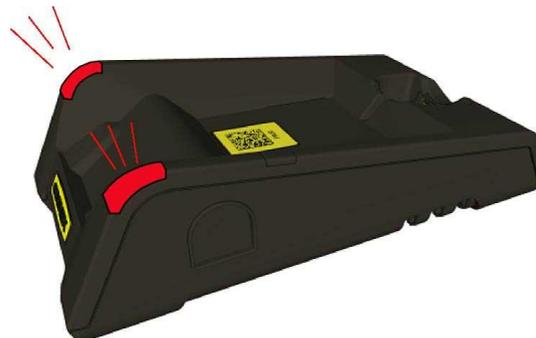
The base station that is paired with a certain reader signals a bad reader alert (beeping and indicators flashing RED) also when another, unassigned reader is put into it.
