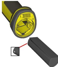
**Note:** Remove the battery from your DataMan 8072 DL before inserting/removing the communication module.
