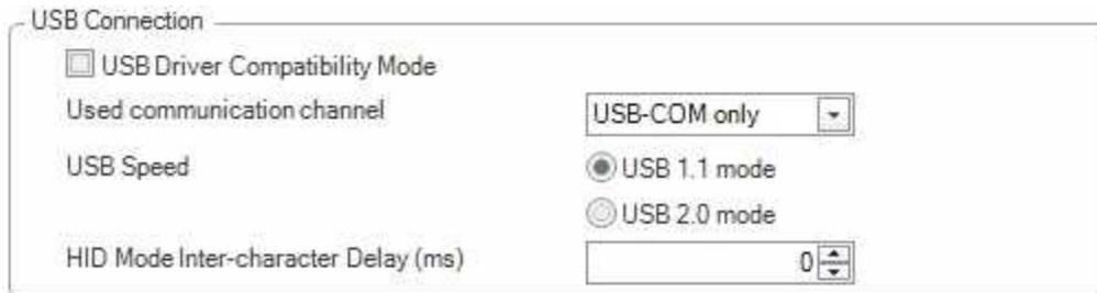
You can also switch the reader and the base station to USB mode (CDC or HID) with a pair of reader configuration codes in the **DataMan Configuration Codes** document.
